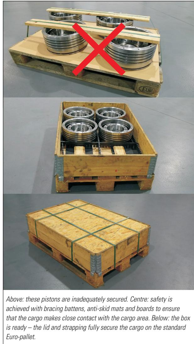
criteria: the cargo should be as close-fitting as possible, it should be placed on anti-skid mats and it should be fastened with a suitable number of straps. In this way it is possible to reduce the risk to a minimum. STI Group is intent on making the subject of cargo security an issue of on-going high priority and, together with its customers, making every effort to ensure that cargo arrives at its destination safely and undamaged.
