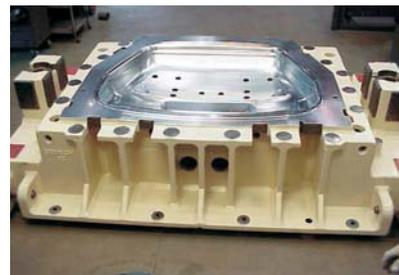
The coated deep-drawing tools result in a significant increase in productivity.
